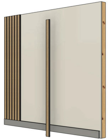
Tongue + groove cladding (loose sticks) traditional install with nails + adhesive
