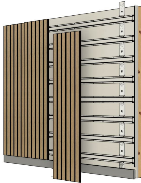
Cambio by Windfall Panels Installed with patented magnetic Wall System
